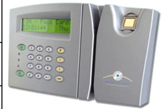
TS7000-BIO Terminal with Magnetic Card and Biometric Reader
